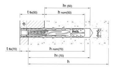
\*\*NOTE\*\* FF1 Anchor system: - The innovative design of the expansion zones enables fixture into AAC blocks with embedment of only 70mm. The FF1 has the flexibility that allows you to define the fixing elements thickness (tfix) value, by adjusting the overall length of your anchor. Example FF1 10x100 has a maximum tfix = 30mm and FF1 10x140 has a maximum tfix = 70mm
